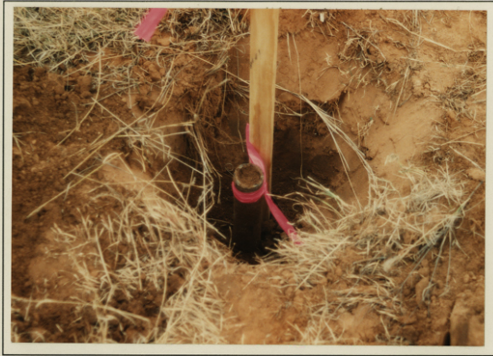
LOOKING DOWN AT A 1-½ INCH IRON PIPE
