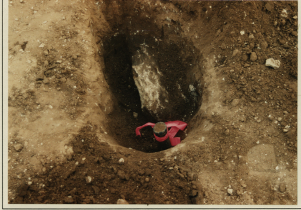
LOOKING DOWN ON A 1-½ INCH IRON PIPE AND STONE
