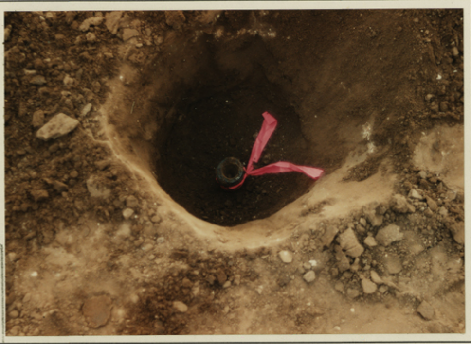
LOOKING DOWN ON 1-1/2 INCH IRON PIPE
