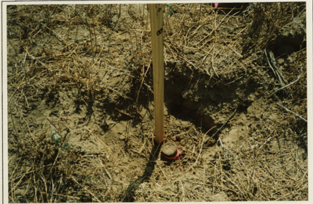
LOOKING DOWN ON A 1-1/4" IRON PIPE
