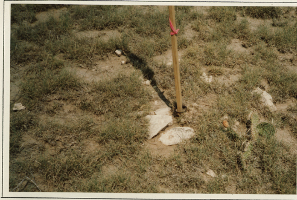
LOOKING DOWN ON A 2" IRON PIPE IN AN OLD ROCK MOUND
