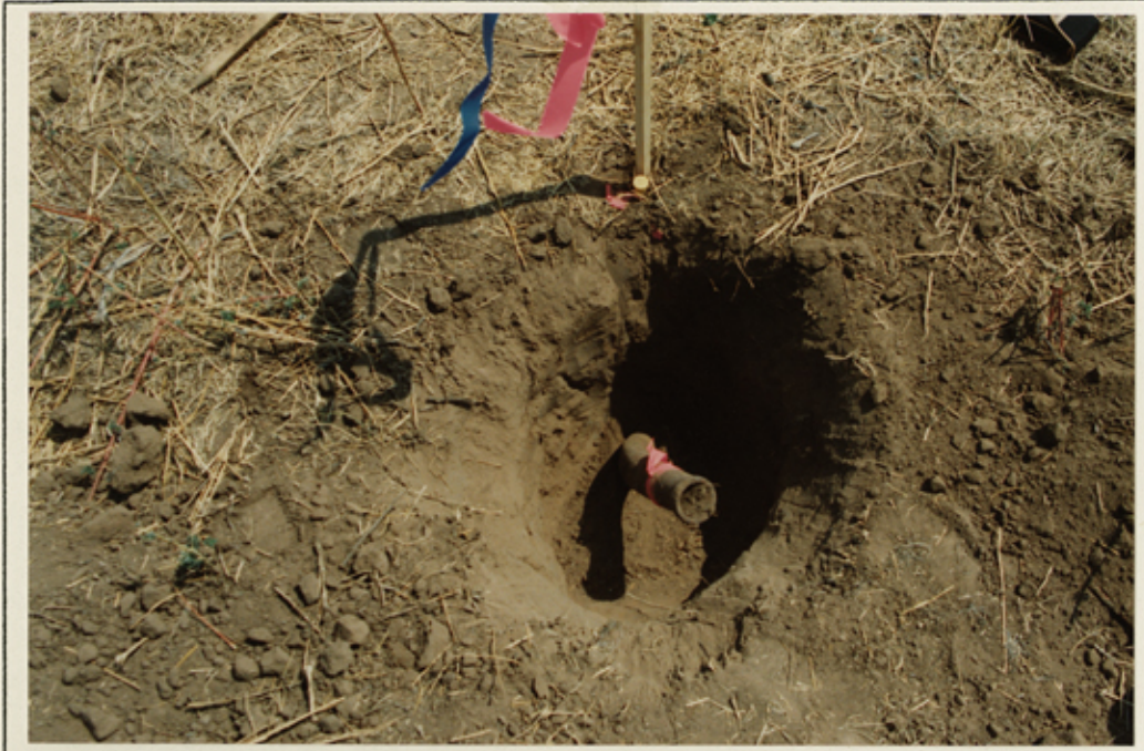
LOOKING DOWN ON A 2" IRON PIPE (BENT) WITH A 1/2" X 30" IRON ROD W/CAP STAMPED "KEYS R.P.L.S. 2507" SET OVER THE BASE OF THE IRON PIPE
