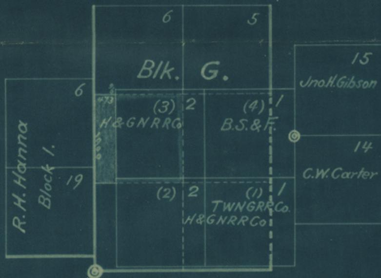
*NOTE:- The corners marked by a double circle on the plat hereon have been identified, as original corners, by State Surveyors R.M. Kenney and Geo. M. Williams.*
