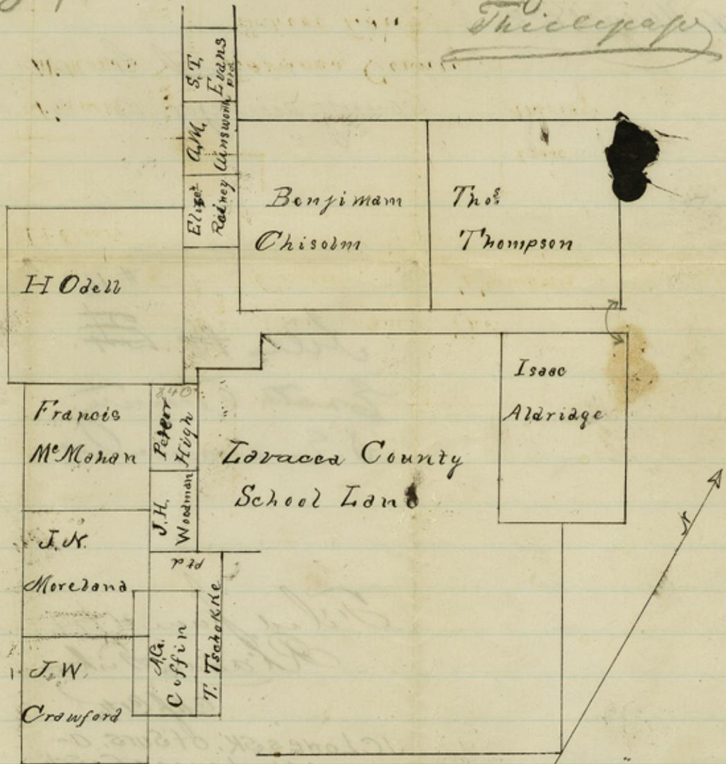
I J C Lowe County Surveyor of Erath County, do hereby certify that the above plat is a true and correct representation of two surveys one made for J. H. Woodman as a home stead. Error in said S. line 10.00 or too long that I have corrected the record to 700.00 being proper distance, on said Woodman survey. The plat is correct representation of the Peter Hugh 148 acre survey, and the field notes of counter 22296
