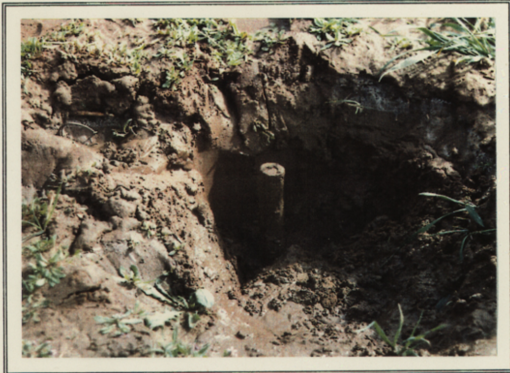
1" X 2' GALVANIZED IRON PIPE AT THE NORTHEAST CORNER OF S. F. 15454 (NO DISCERNIBLE MARKINGS)
