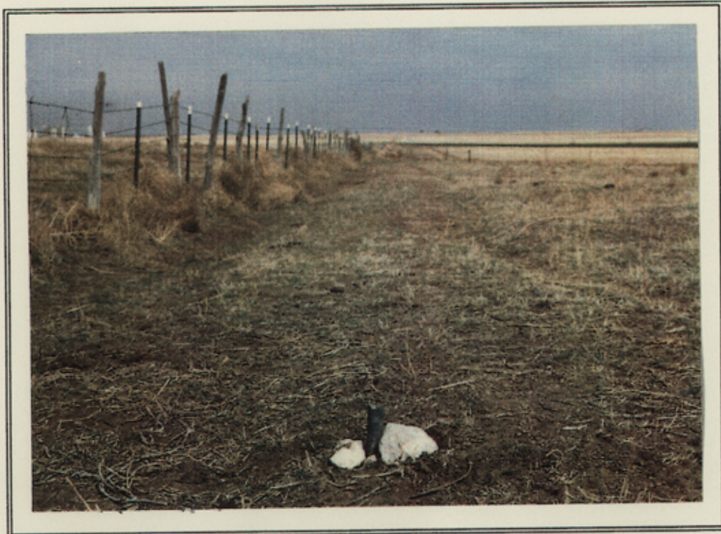
1-1/4" GALVANIZED IRON PIPE, TOP BROKEN OFF, AT THE NORTH COMMON CORNER OF SECTIONS 136 AND 165; LOOKING EAST
