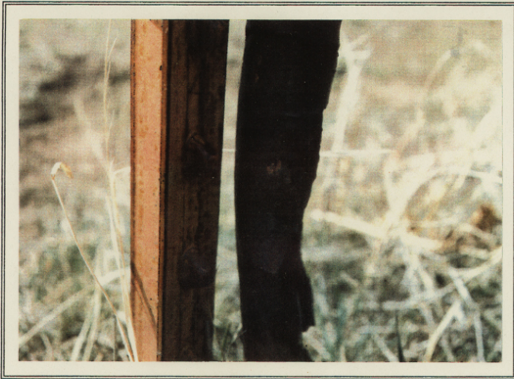
1" IRON PIPE AT THE NORTH COMMON CORNER OF SECTIONS 17 AND 18; EAST SIDE OF PIPE STAMPED "18"
