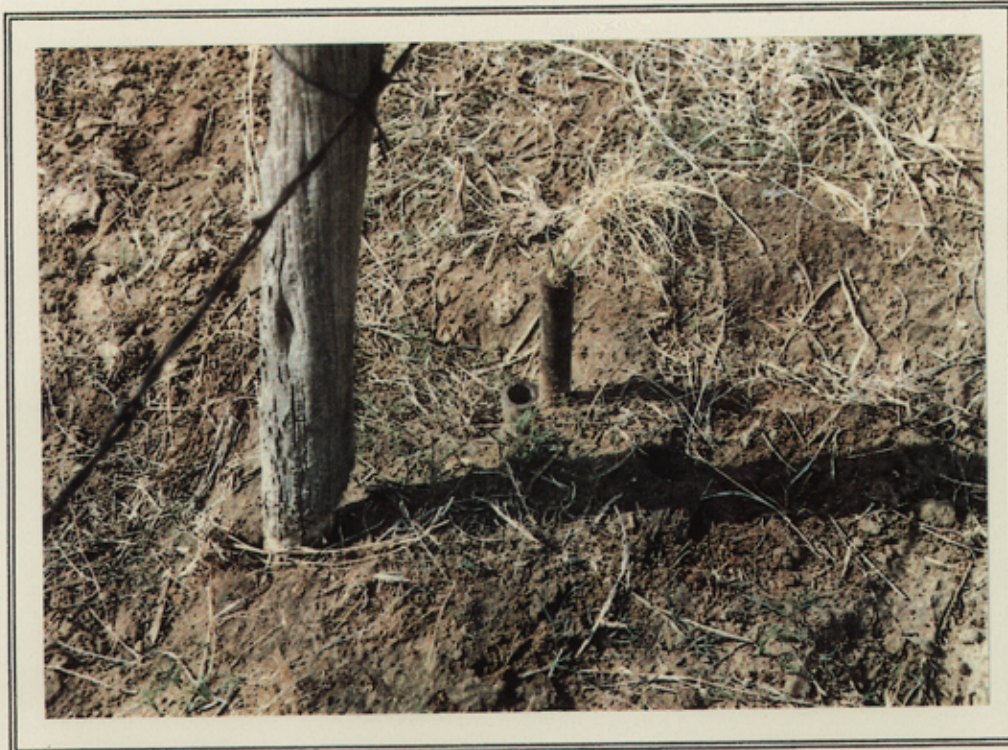
TWO 1/2" IRON PIPES AT THE NORTH COMMON CORNER OF S. F. SURVEYS 15481 AND 15456
