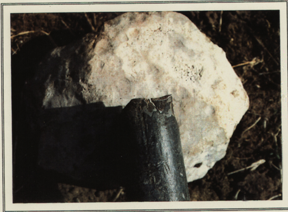
1-1/4" GALVANIZED IRON PIPE, TOP BROKEN OFF, AT THE NORTH COMMON CORNER OF SECTIONS 136 AND 165; STAMPED "17 - 165"
