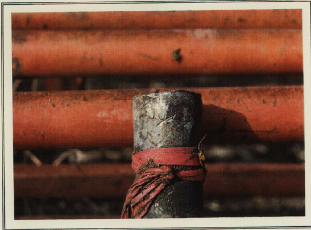
1-1/4" GALVANIZED IRON PIPE AT THE COMMON CORNER OF SECTIONS 106, 107, 134 AND 135; STAMPED "106-107-134-135"
