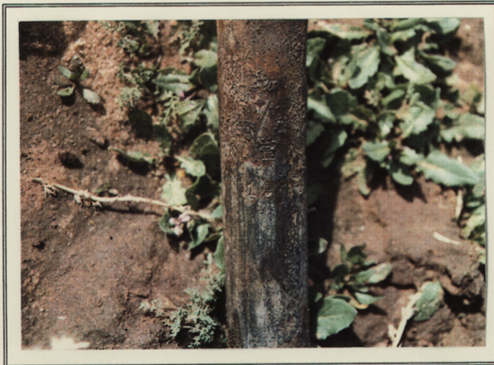
1" X 3' GALVANIZED IRON PIPE AT THE NORTH COMMON CORNER OF SECTIONS 19 AND 20; STAMPED "NE 19"
