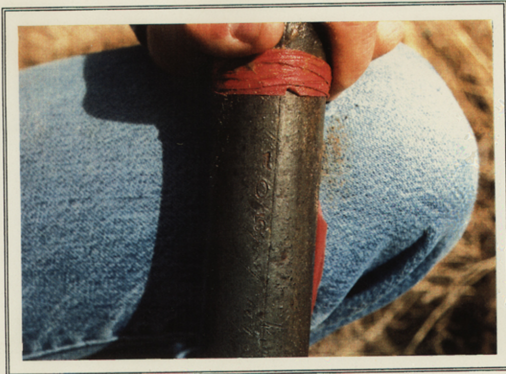
1-1/4" X 2' GALVANIZED IRON PIPE AT THE SOUTH COMMON CORNER OF SECTIONS 20 AND 21; STAMPED "20-21-105"
