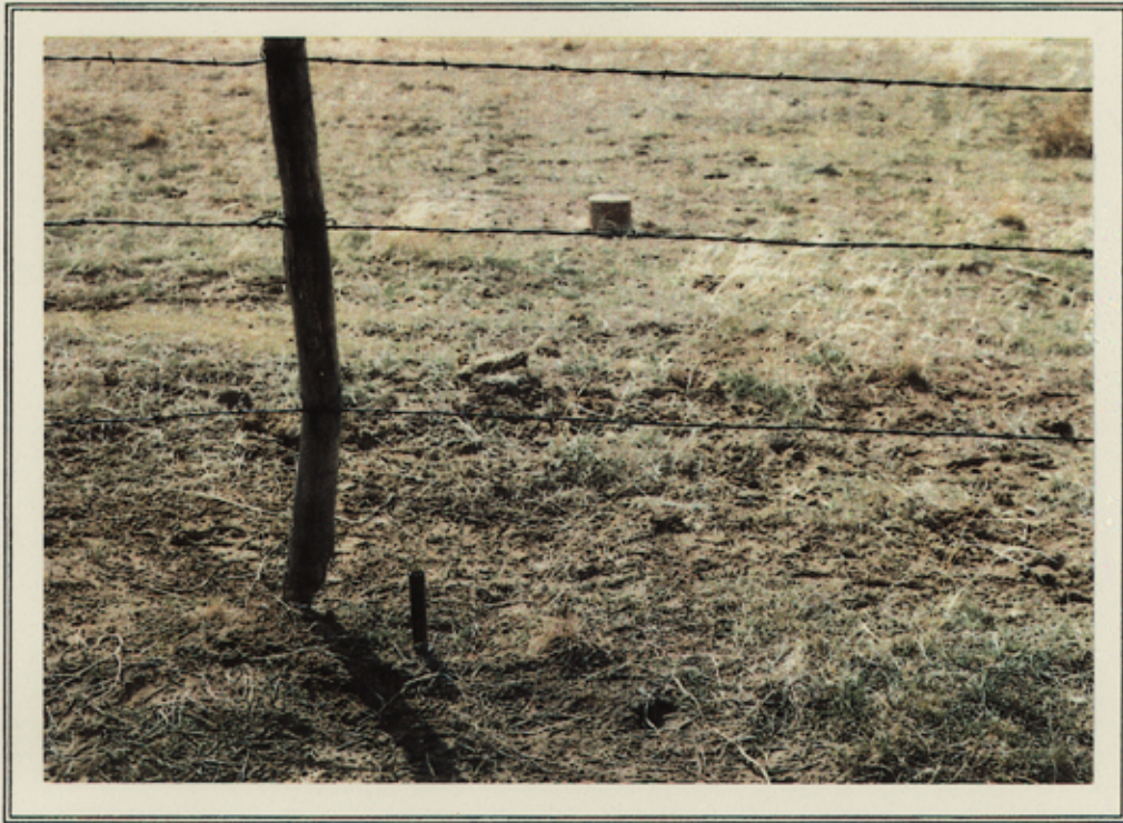
TWO 1/2" IRON PIPES AT THE NORTH COMMON CORNER OF S. F. SURVEYS 15481 AND 15456; LOOKING WEST (U. S. G.L.O. MONUMENT IN BACKGROUND)
