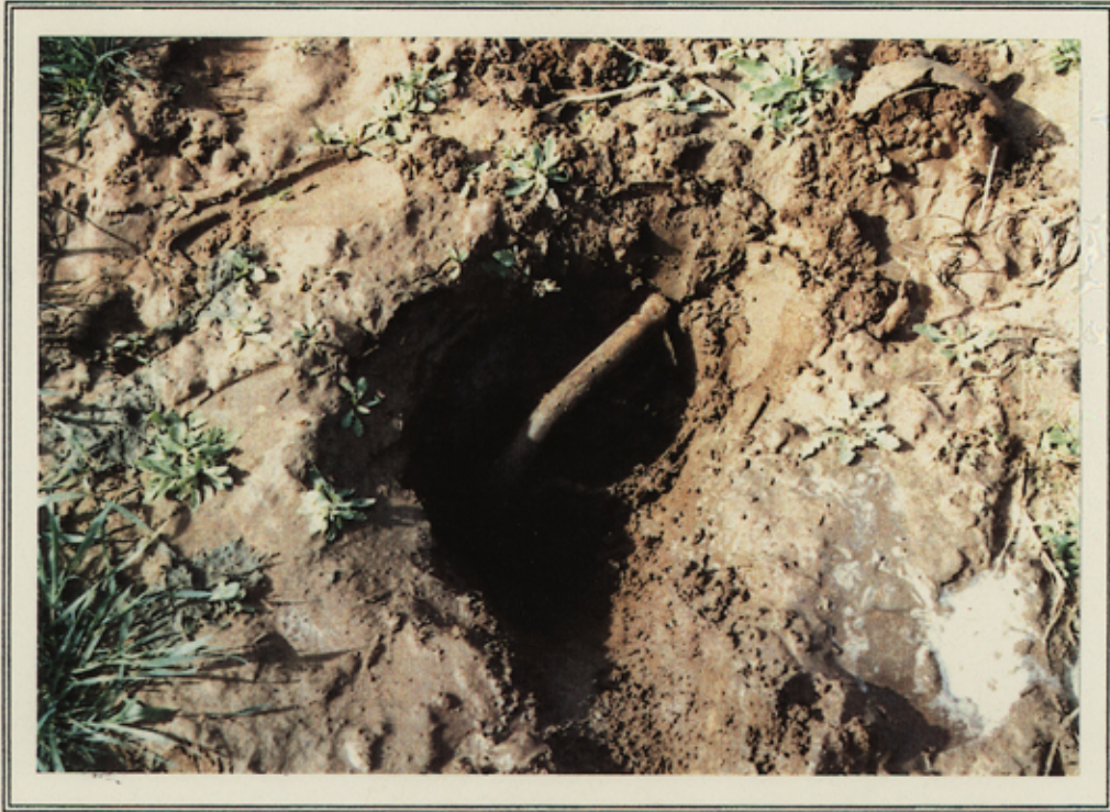
1" X 3' GALVANIZED IRON PIPE AT THE NORTH COMMON CORNER OF SECTIONS 19 AND 20
