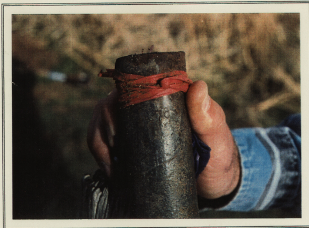
1-1/4" GALVANIZED IRON PIPE AT THE NORTH COMMON CORNER OF SECTIONS 76 AND 105; STAMPED "21-76-105"
