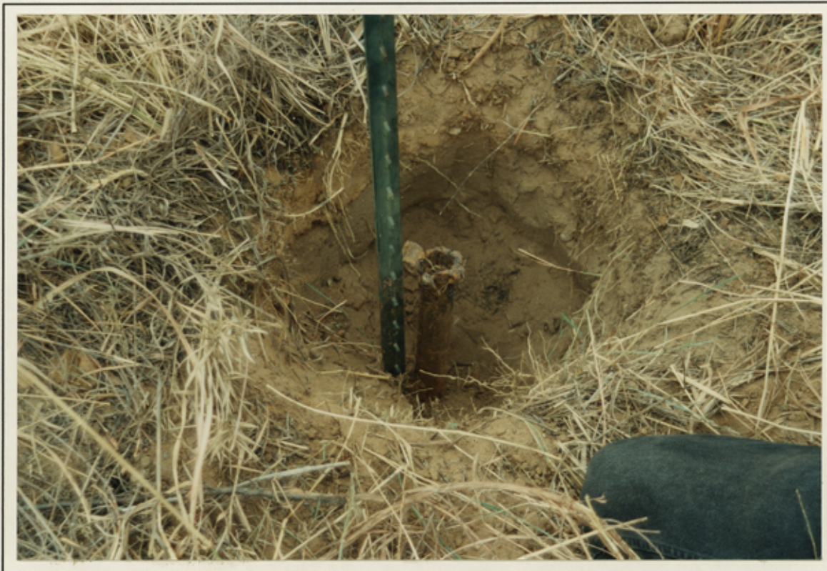
DETAIL OF 1-1/2" IRON PIPE AT COMMON CORNER OF SECTIONS 21, 22, 39 AND 40, BLOCK A3, H. & G. N. RR. CO. Wheeler sk. File 11
