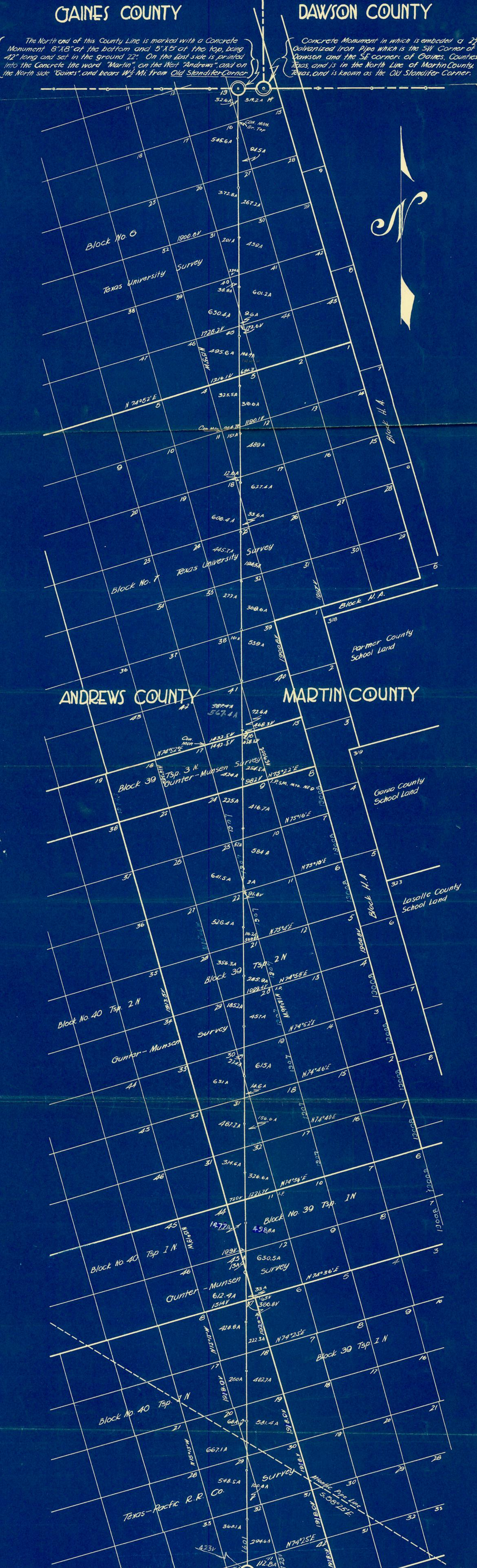
Concrete Monument 8"X8" at the bottom and 5"X5" is printed in Concrete the word Andrews, on the E. side the word "Marting and on the south side, the word "Midland" This monument bears W. 7 m. from point where the Estes corner was, as called for in judgment in establishing this line; also the 25 Mi. post in Midland Co. N. line bears E. 1048.8 Vrs., being
