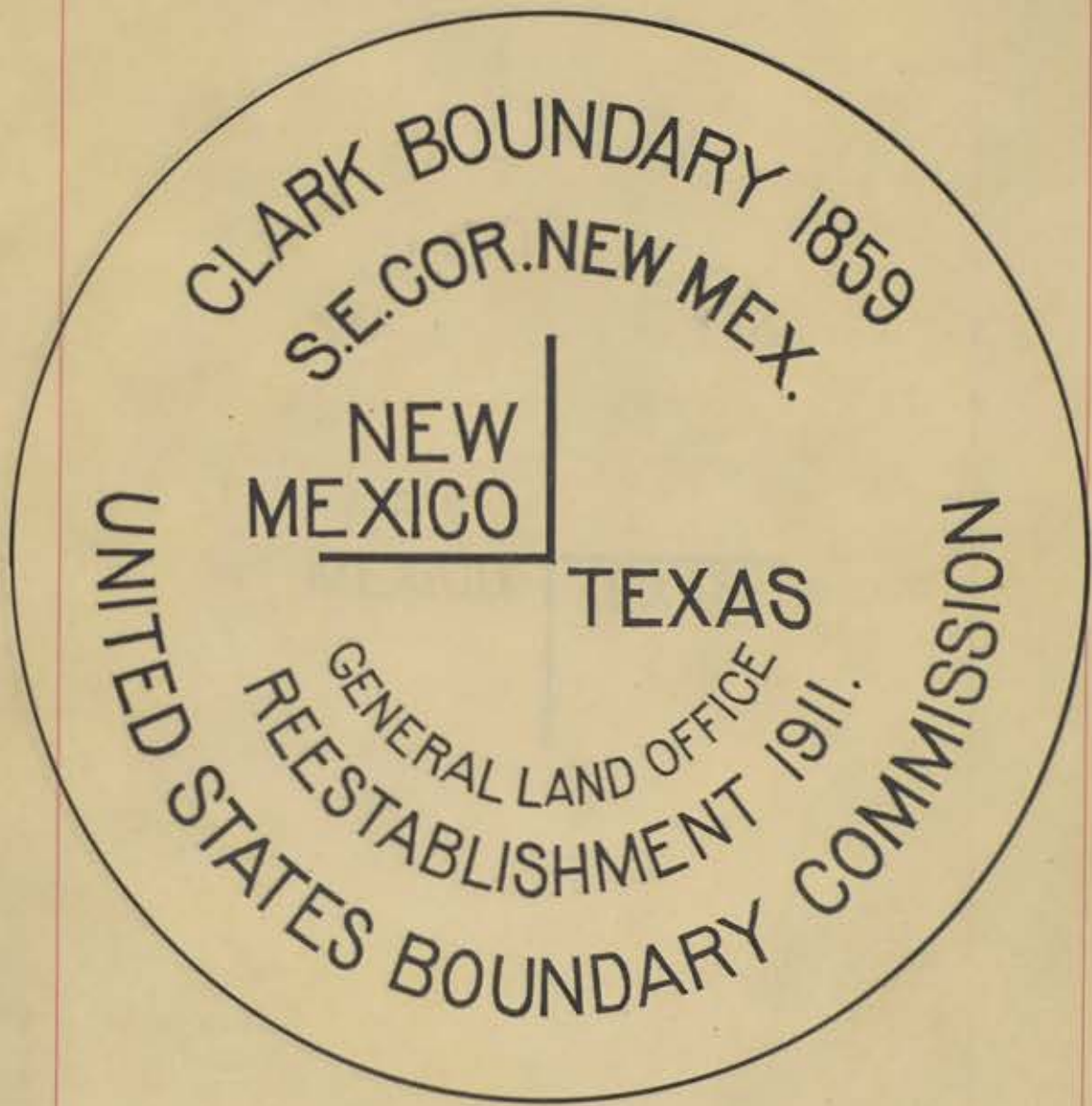
Diagram of plate imbedded in concrete monument at S.E. corner of New Mexico, actual size.
