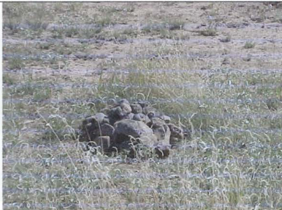
MVC 791f – Rebuilt Mound In Position Of L.E. Edwards, Original Common Cor Of Sec. 547,576,577 & 578, Blk. 8
