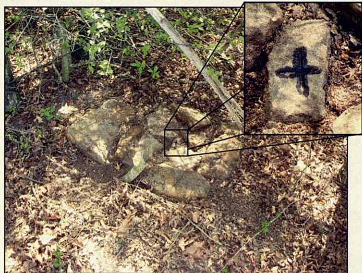
Figure 1: Set stone found in rock mound for the west corner of the William G. Lilley Survey. Inset: set stone marked "X".
