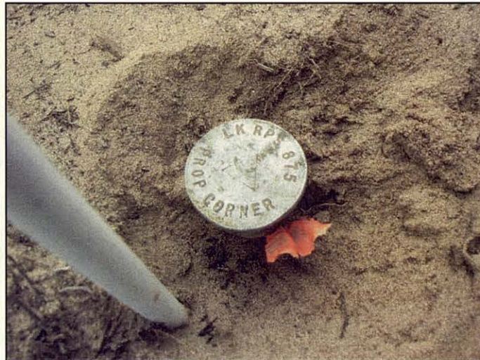
Figure 4: Iron Rod found with aluminum cap stamped "LK RPS 875 PROP CORNER" for the southeast corner of the Remaining Part of the William G. Lilley Survey.
