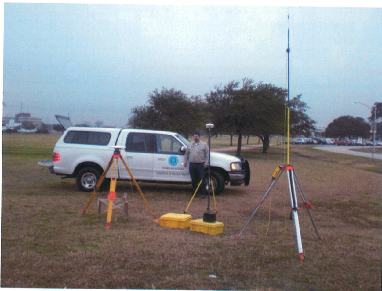
Fig. 14. Workhorse of the Camp Mabry boundary survey was GPS and a truck. Left foreground: Trimble R7 GNSS dual frequency receiver and Zephyr Geodetic2 antenna with ground plane set up over Station 500, used as the Base. Right foreground: Trimble TRIMMARK-3 base station radio and antenna used as the VHF communication link to send relative-positioning corrections to the Rover receiver. Middle foreground: Trimble R6 GNSS dual frequency receiver on a 2-meter fixed composite rod with Trimble TSC2 Survey Controller data collector, used as the Rover. Mark Hinojosa poses in the background. View looking south at the Parade Field on Camp Mabry.
