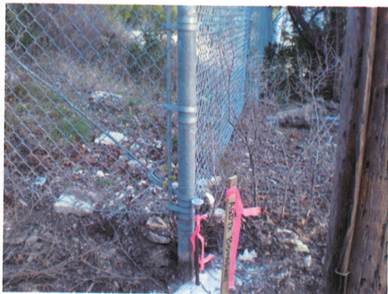
Fig. 11. Point of Beginning: A 5/8" iron rod with aluminum cap stamped AGDTX-BOUNDARY set for corner at the southwest base of a steel chain link fence corner post at the intersection of the present northeast Right-of-Way line of West 35 th Street and the southeast line of Lot 1, Block 1, Colorado Foothills Section One. View is looking southeast.
