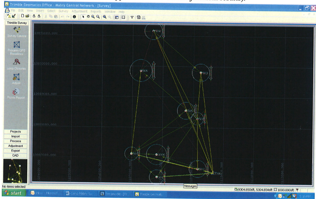
Fig. 3. Geodetic control network established on Camp Mabry, 30 September 2009. Colored bars for the error ellipses over the points represent measured statistical horizontal and vertical errors in +/- 0.01-foot increments. Gray dotted lines represent a grid overlay of 1,000-foot squares.
