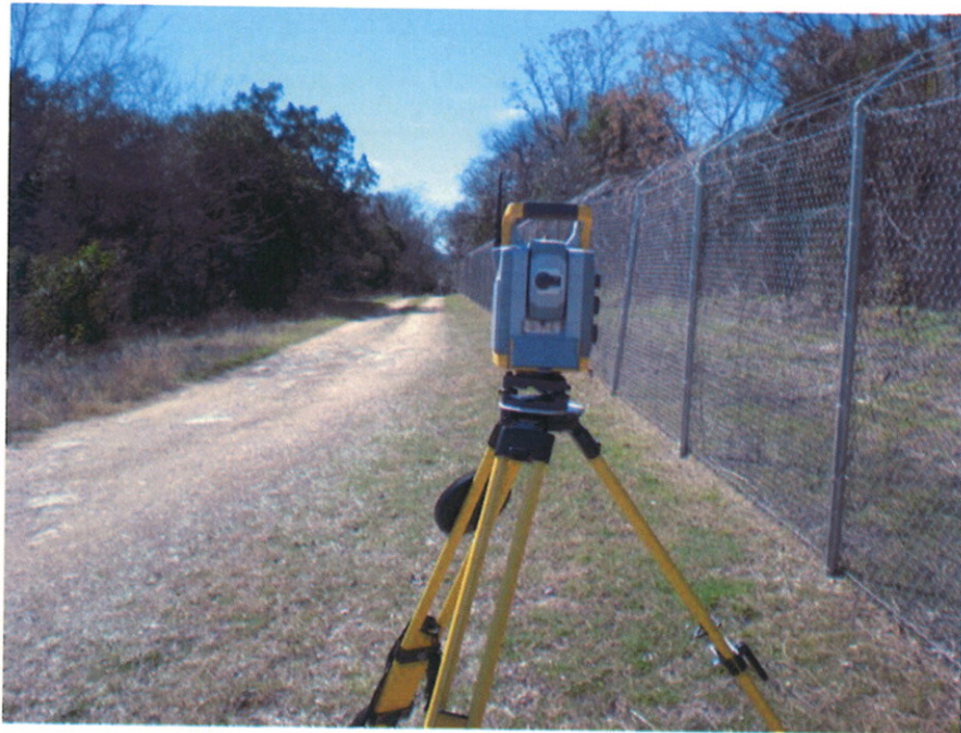
Fig. 7. Trimble S6 total station robot locked on to a prism rod taking a back sight. The antenna on the robot receives commands from the data collector controlled by the operator (at the prism rod) and sends data back for logging. In this configuration, the robot tracks the prism rod's infrared beacon, and measures distances with infrared. The Direct Reflectorless mode uses a laser beam pointed at the object that is being measured and does not require use of the prism rod. This location is near the northwest corner of Camp Mabry. The chain link fence is the security fence constructed after 911.
