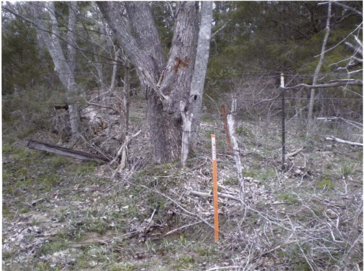
Figure 8. Set corner at east line of Camp Maxey and northeast line of the Town of Powderly. A 24-inch elm tree with blazed "X" bears North 53^{\circ}47' 7.3 feet (David A. Rolbiecki, RPLS).
