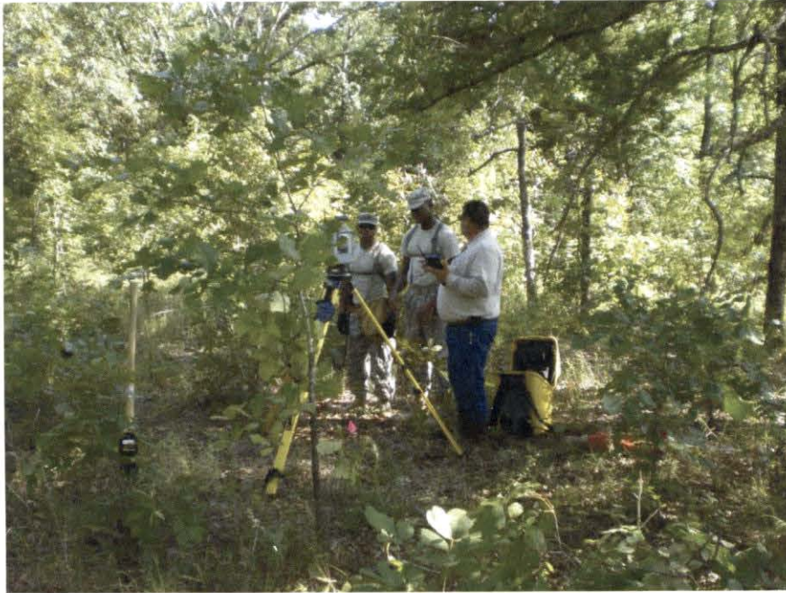
Mark Hinojosa, Specialist Daruis Baylor and Specialist Torrance Bowman with Trimble S6 traversing along the north line of Parcel-I, July 2012 (David A. Rolbiecki, RPLS).
