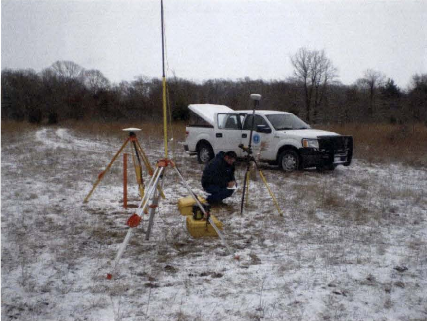
Mark Hinojosa setting up Trimble R7 GNSS base receiver, Zephyr Model-2 geodetic antenna and Trimmark-3 base radio transmitter/receiver at Station 500 January 2013 (David A. Rolbiecki, RPLS).
