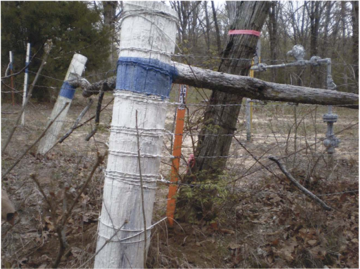
Figure 6. Ancient wooden fence corner post found for northwest corner of the Town of Powderly (looking southeast). A 60D nail flagged pink can be seen about a foot above the ground. White and blue-painted gas easement fence post seen in foreground bears North 20°14' West 2.9 feet (David A. Rolbiecki, RPLS).
