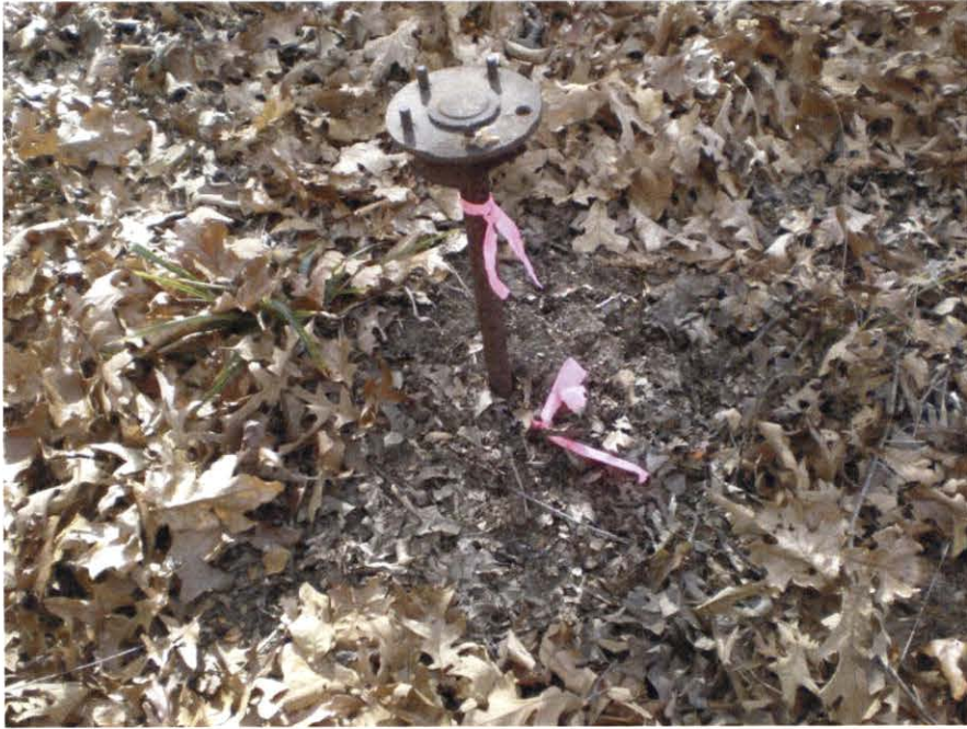
1/2" iron rod found next to car axle at NEC Caldwell 1.45 acre Land Exchange (David A. Rolbiecki, RPLS).
