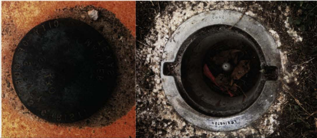
Figure 2: City of Corpus Christi monument 'SK-130' and NGS monument 'LEXINGTON' were used as horizontal control for the coastal boundary survey at North Beach, Corpus Christi.
