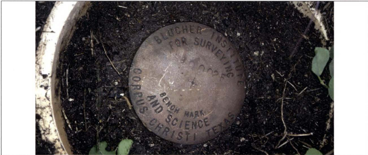
Figure 2: NGS monument '90002 F' was used as horizontal and vertical control for the coastal boundary survey at McGee Beach, Corpus Christi.
