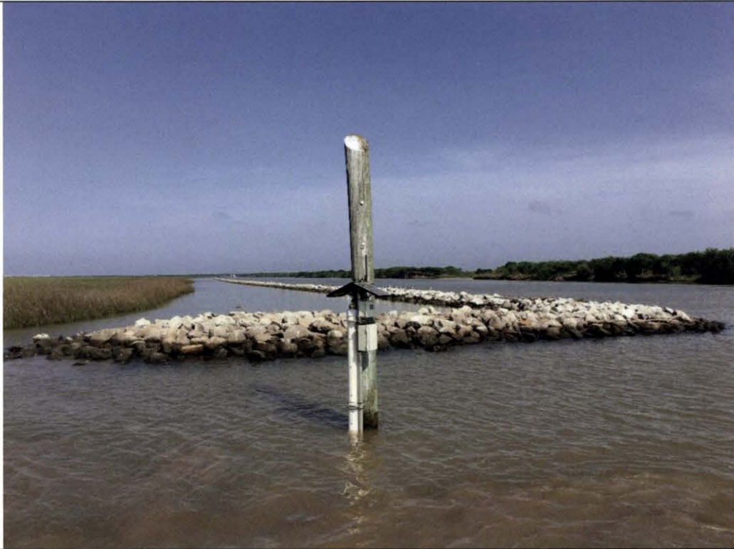
Figure 2: Onsite (station) tide gauge setup on a piling alongside the GIWW on existing breakwater adjacent the north GIWW shoreline of Mad Island.
