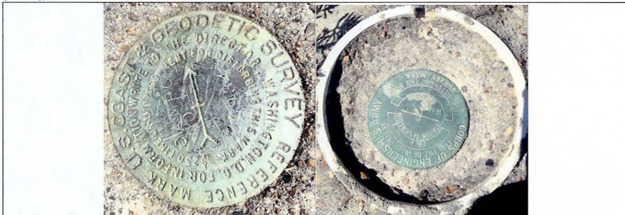
Figure 1: NGS monument "CAMPO REF1 1934", left, was used as horizontal and vertical control for the coastal boundary survey along the Matagorda Bay shoreline; USACE benchmark "EO Y" was used to tie in onsite tide gauge, right.
