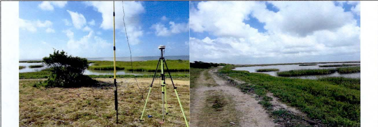
Figure 4: An onsite TBM was used for local control and GPS RTK base setup, left; typical onsite vegetated shoreline and marsh landward of the MHHW line.
