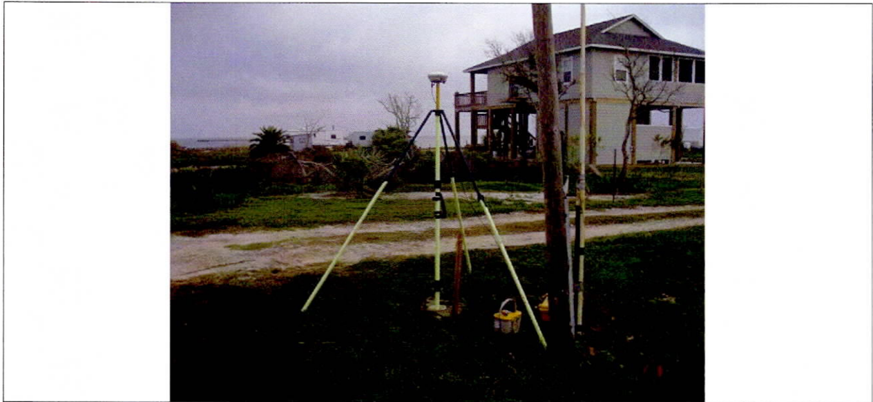
Figure 2: tidal reference monument "LUB 0971 D 1994" was used as horizontal and vertical control for the coastal boundary survey along the Gulf coast of Bolivar Peninsula
