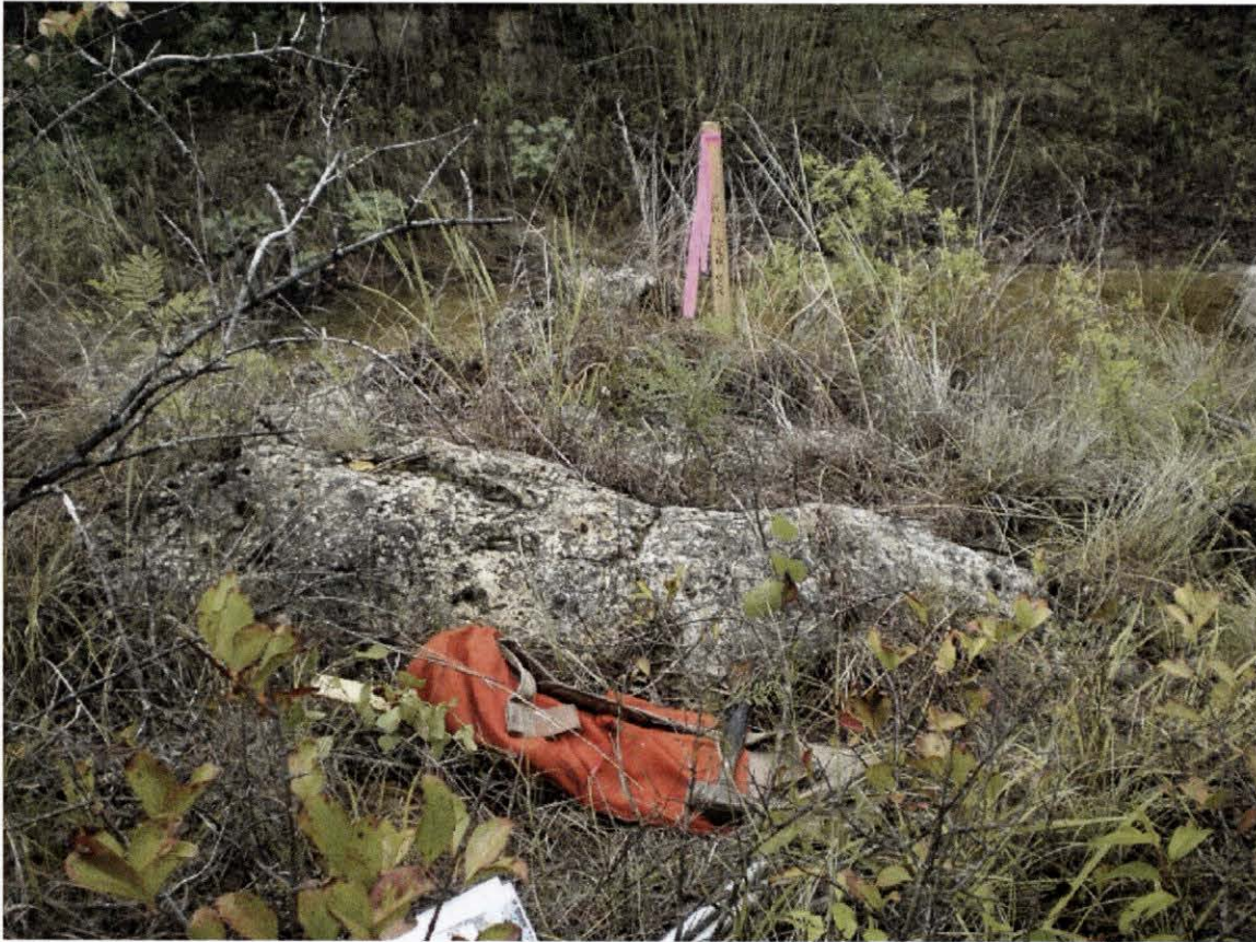
Figure 13. Found rock on top of west bank of Moss Branch for NE corner of the P.H. Pope Survey.
