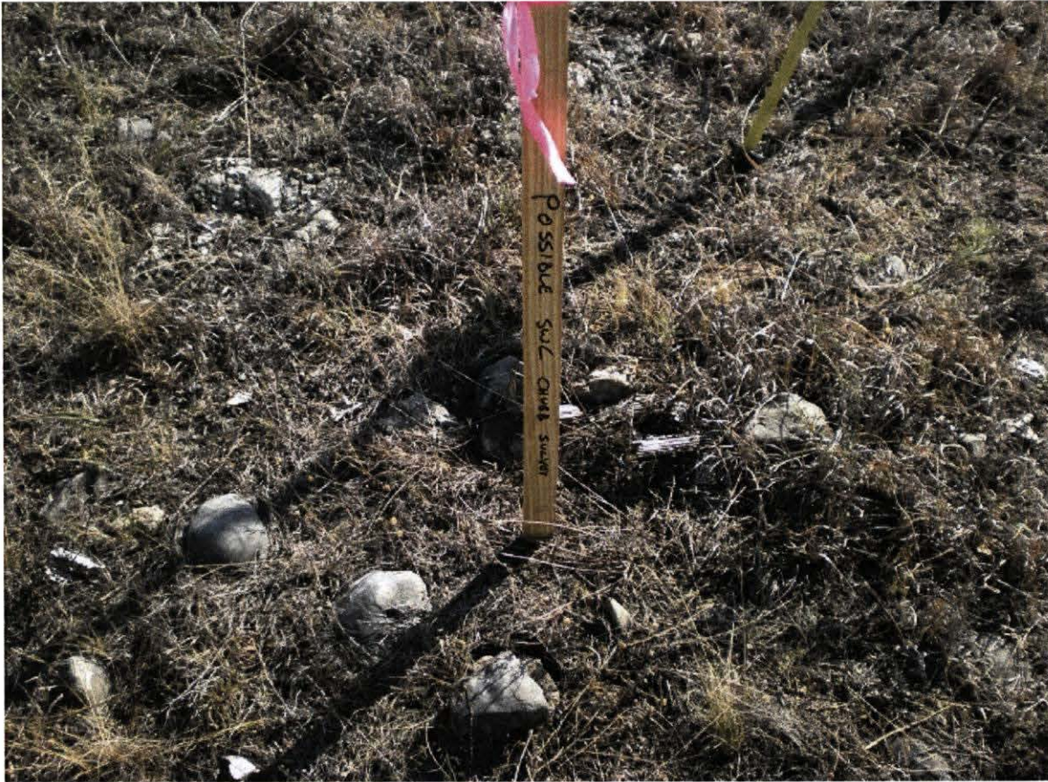
Figure 2. Found circle of rocks for the SE corner of the Thomas Chubb Survey.
