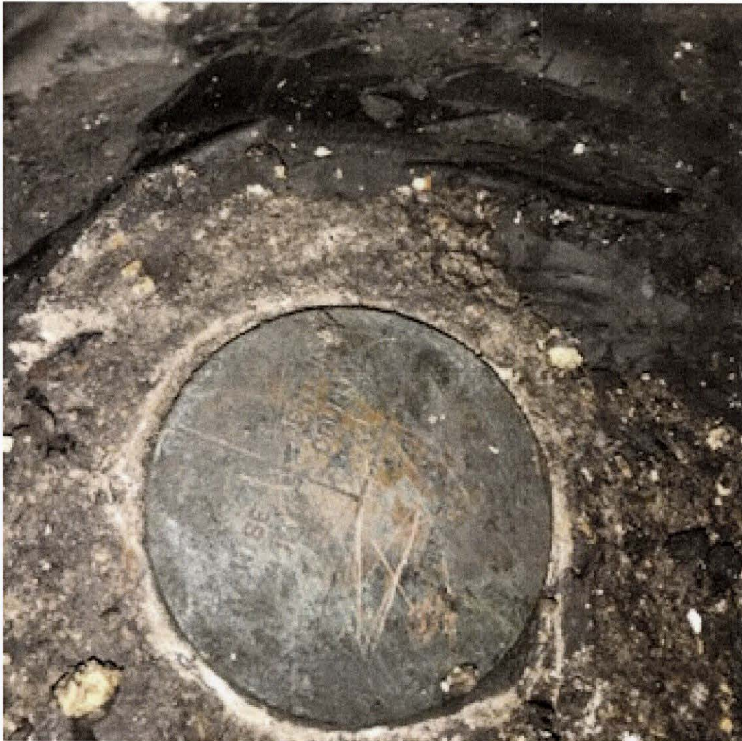
Figure 6. Found brass disc in concrete for the common corner of Wise, Denton and Tarrant Counties set by Garey Gilley, RPLS, LSLs during his survey of the Tarrant-Denton County line from December 2004 to June 2005.
