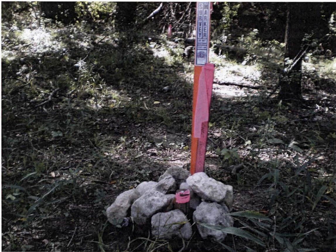
Figure 3. Reconstructed corner common with the George McCloud, Wm. G. King, Thomas Chubb and J.P. Smith Surveys. This I made a point of intersection on the south boundary line of Eagle Mountain Lake TRACT 1. The T.J. Elkins found 1-inch iron rod on the north bank of Indian Creek is seen in the background to the south.
