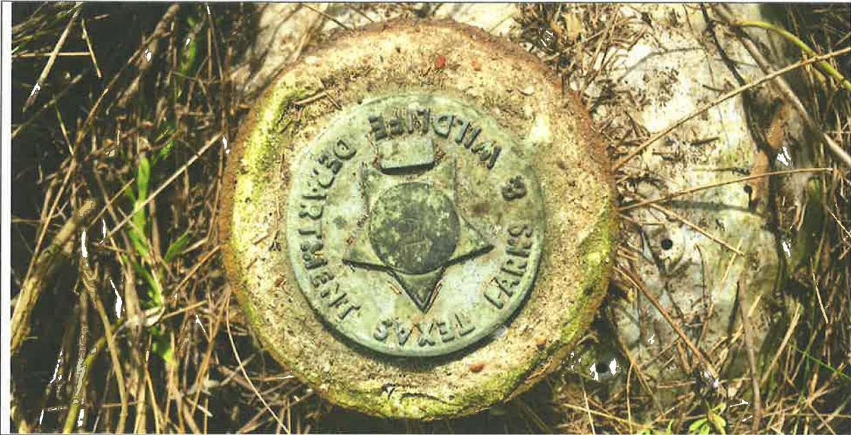
**Figure 5:** The east end point of the MHW line (littoral boundary) was tied to a refuge corner which was marked with a bronze TPWD monument set in a cast iron pipe (N:13,824,938.66, E: 3,533,646.37, EL: 2.9')
