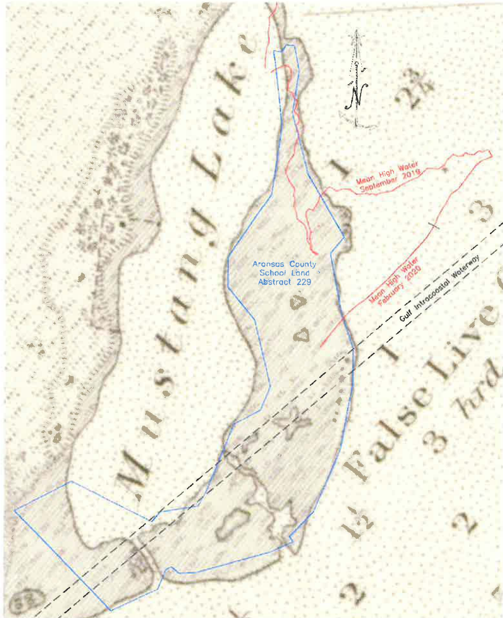
Figure 5: The current (September 2019, February 2020) MHW (red), original Aransas County School Land Survey No. 68, Abstract 229 (February 1878, blue) and Gulf Intracoastal Waterway overlaid on 1884 Coast and Geodetic Survey Coast Chart No. 108 of Pass Cavallo, Lavaca and San Antonio Bays
