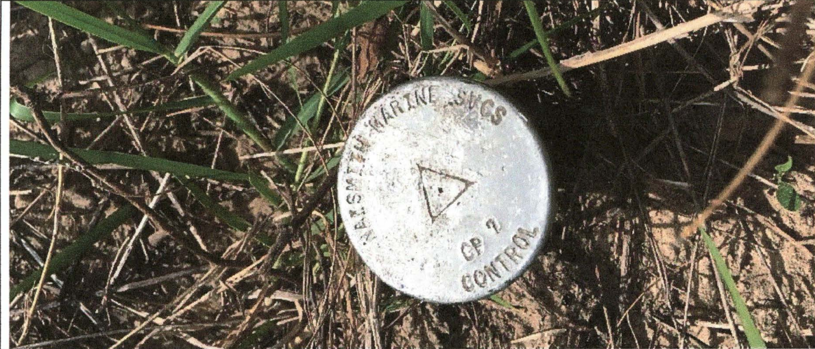
Figure 3: Typical TBM set during the survey was a 3/4" galvanized iron pipe with an aluminum cap stamped "NAISMITH MARINE SVCS CONTROL". "CP2" was set at the east end of the project (N:13,823,472.48, E: 3,533,731.28, EL: 7.0')
