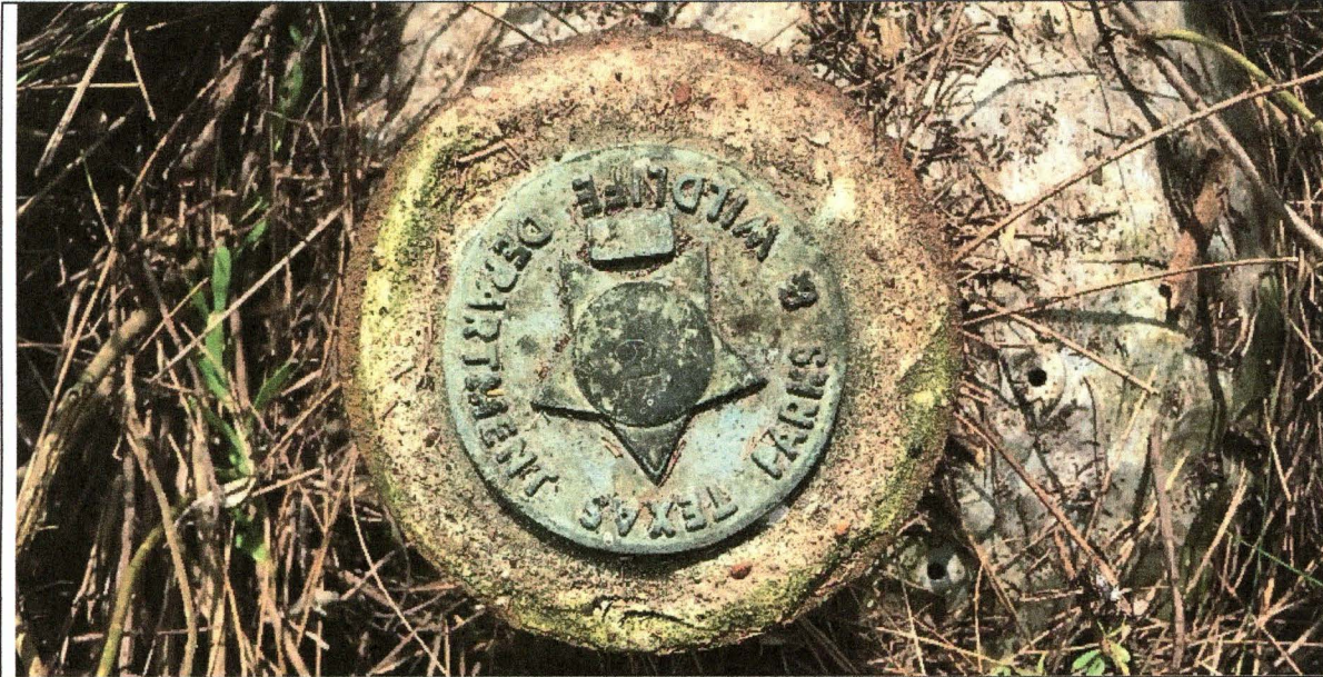
Figure 5: The east end point of the MHW line (littoral boundary) was tied to a refuge corner which was marked with a bronze TPWD monument in a cast iron pipe (N:13,824,938.66, E: 3,533,646.37, EL: 2.9')
