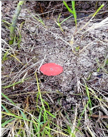
Figure 5: 5/8" iron rod found with red cap set by J.L. Brundrett, Jr. noted in NRC Article 33.136 Sketch 9 (N: 13,236,724.43, E: 2,618,845.91, EL: 2.40 NAVD88)
