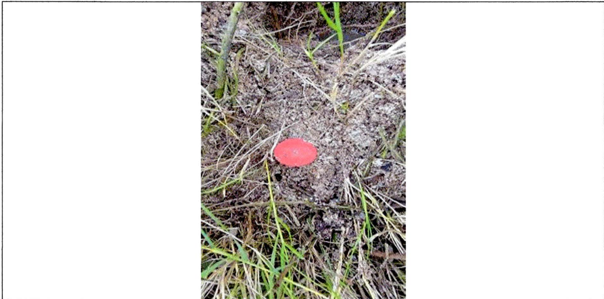
Figure 3: 5/8" iron rod found with red cap, set by J.L. Brundrett 09 April 2013 noted in Article 33.136 Sketch 9 (N: 13,236,724.43, E: 2,618,845.91, Elev: 2.4' NAVD88)
