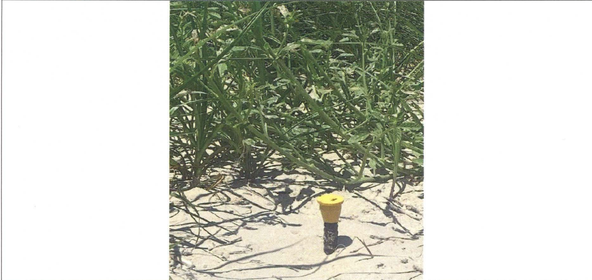
Figure 5: 5/8" iron rod set with yellow cap "TBS" (N: 13,657,628.41, E: 3,283,197.27, EL: 6.6' NAVD88)
