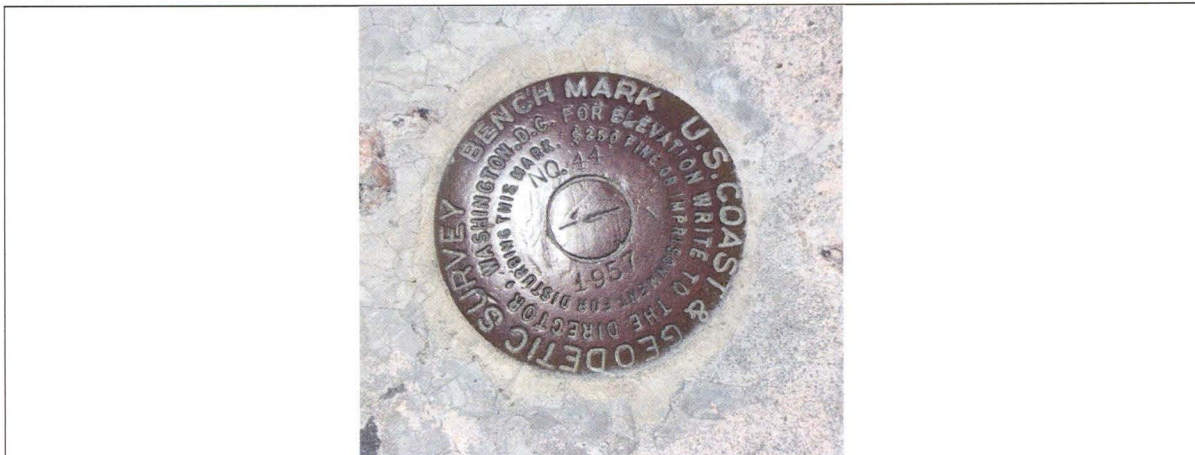
Figure 2: NGS benchmark "877 1510 TIDAL 44" (N: 13,676,511.25, E: 3,310,080.49, EL: 14.45' NAVD88) Shared OPUS Solution
