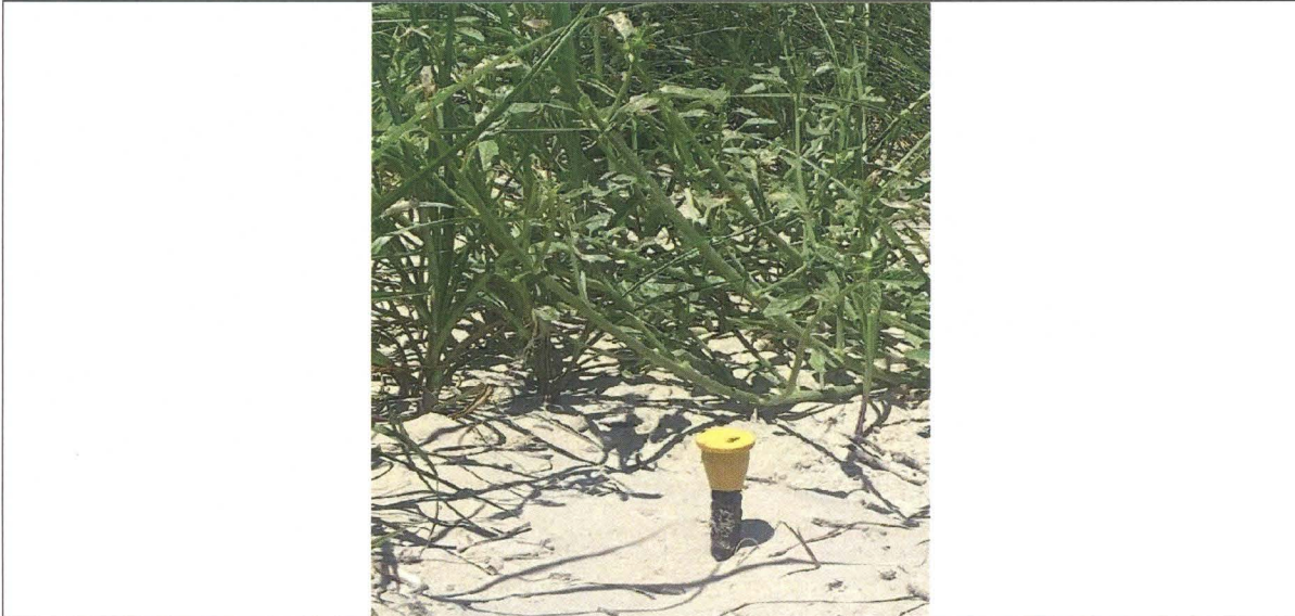
Figure 3: 5/8" iron rod set with yellow cap "TBS" (N: 13,657,628.41, E: 3,283,197.27, EL: 6.6' NAVD88)
